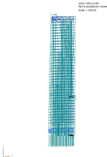
Figure 3.12: Tall building with stiff core.
