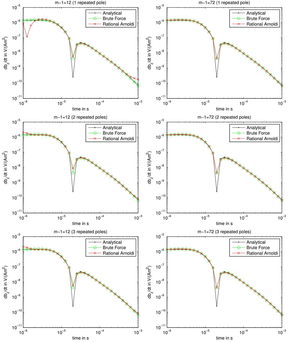
**Figure 3.** Comparison of transients  $\partial_t B_z$  evaluated at  $\mathbf{x} = (100, 0, 0)$  m extracted from a rational Arnoldi approximation of order  $m = 13$  and  $m = 73$  (left and right columns, resp.) using 1, 2, and 3 cyclically repeated poles (top, middle, and bottom row, resp.) with an analytical solution, and the brute force solution obtained by inverse Fourier transform of frequency-domain solutions (14) for the layered half-space model. Nédélec FE of order  $k = 1$ .
