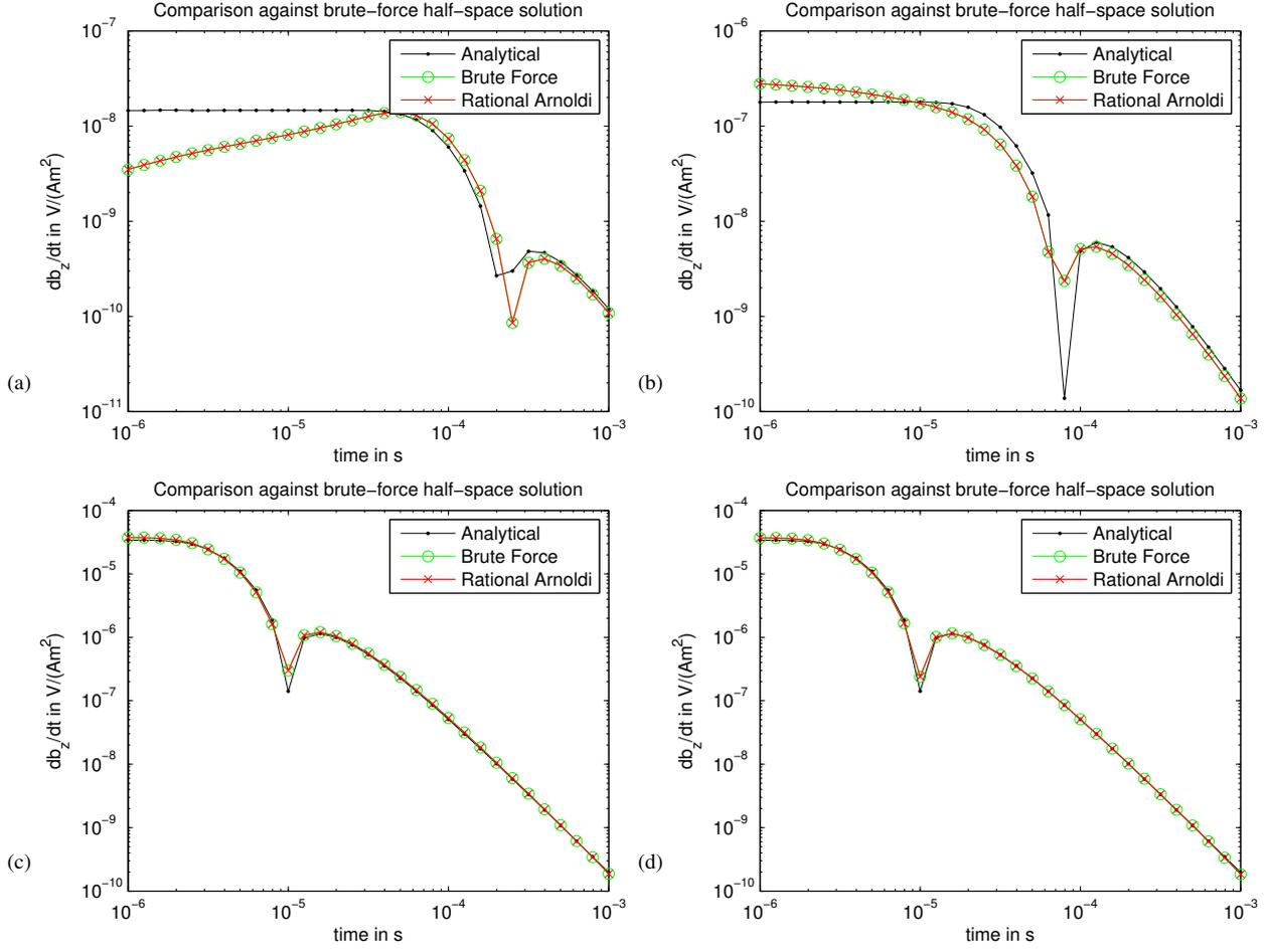
**Figure 8.** Comparison of transients  $\partial_t B_z$  computed from a rational Arnoldi approximation of order  $m = 36$  with an analytical solution, and a brute force solution obtained by inverse Fourier transform of frequency-domain solutions for the topography model, Nédélec elements of order  $k = 2$ , taken at the plane  $y = 0$  at points  $x = [-130, 0, 130, 270]$  m, and  $z = [0, 38, 0, 0]$  m. The  $20 \times 20$  m<sup>2</sup> transmitter loop source is centered at  $x = 200$  m.
