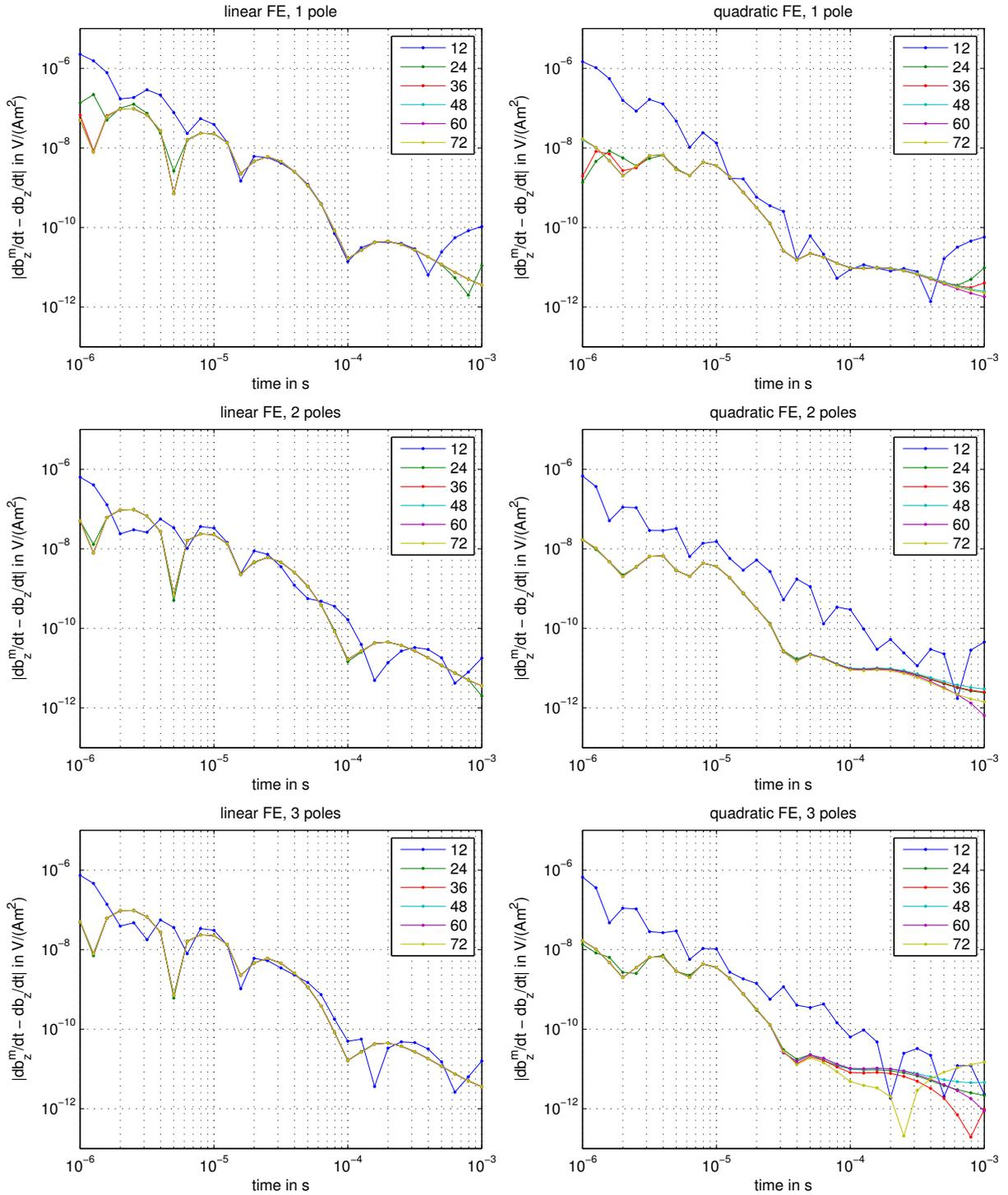
**Figure 5.** Absolute error between the transient  $\partial_t B_z$  evaluated at  $\boldsymbol{x} = (100, 0, 0)$  m extracted from rational Arnoldi approximations with  $m - 1 = 12, 24, \dots, 72$  and the transient obtained by the analytical solution for the layered half-space.
