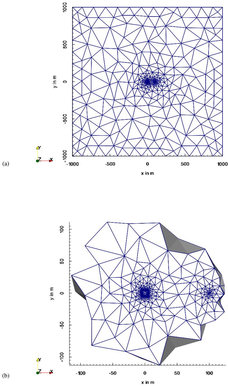
**Figure 1.** Trace of the tetrahedral finite element mesh on the plane  $z = 0$  (a). Panel (b) zooms into the area of transmitter and receiver. The air layer, which has a thickness of 1000 m, has been omitted in the plots.
