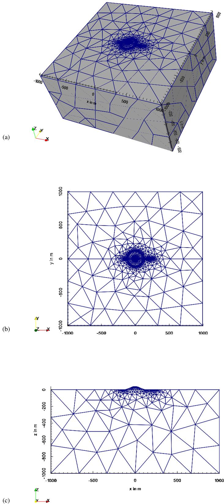
**Figure 7.** Trace of the tetrahedral finite element mesh used for computation of the transients: Perspective view (a), view from above onto Earth's surface (b), vertical slice along the plane  $y = 0$  (c). The air layer, which has a thickness of 1000 m, has been omitted in all pictures.
