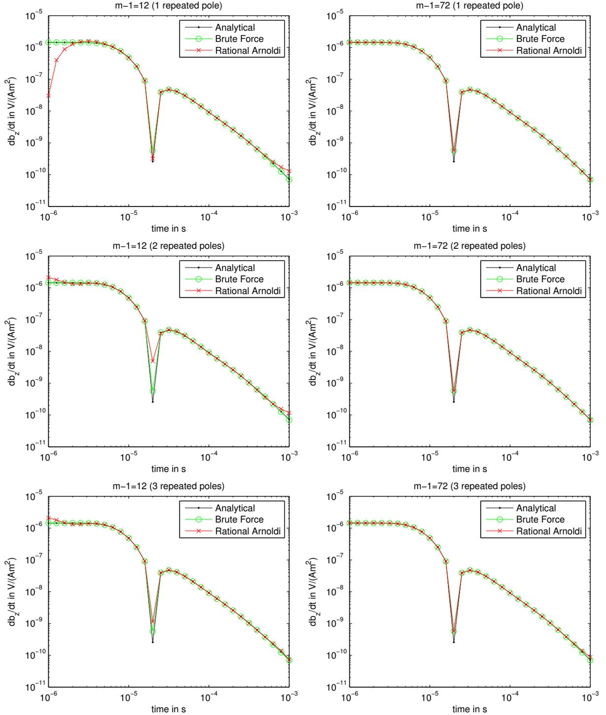
**Figure 4.** Comparison of transients  $\partial_t B_z$  evaluated at  $\mathbf{x} = (100, 0, 0)$  m extracted from a rational Arnoldi approximation of order  $m = 13$  and  $m = 73$  (left and right columns, resp.) using 1, 2, and 3 cyclically repeated poles (top, middle, and bottom row, resp.) with an analytical solution, and the brute force solution obtained by inverse Fourier transform of frequency-domain solutions (14) for the layered half-space model. Nédélec FE of order  $k = 2$ .
