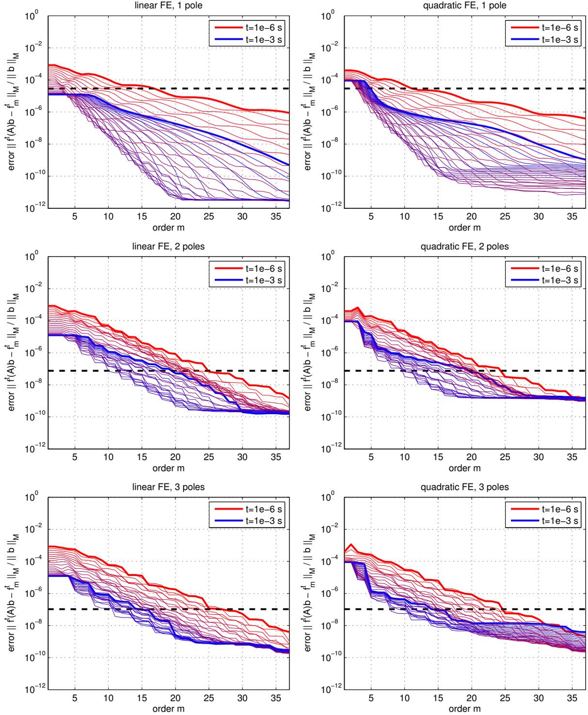
**Figure 2.** Errors of the rational Arnoldi approximations of dimension  $m = 1, 2, \dots, 37$  with respect to a higher order rational Arnoldi approximation ( $m = 42$ ) for all desired times  $t \in [10^{-6} \dots 10^{-3}]$  s, where the poles used are those optimized for  $m - 1 = 36$ .
