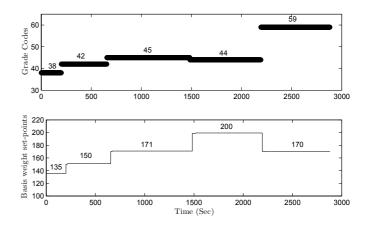
Fig. 3. Grade codes (top) and basis weight set-points (bottom) scheduled by the mill
