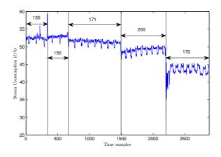
Fig. 6. Actual steam consumption for each grade 5.2 Example 2: Scheduling Multiple Orders
