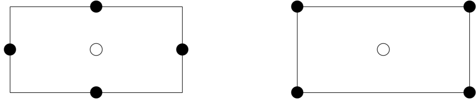
Figure 4.8: The left and right pictures are the degrees of freedom for the rotated and the standard Q_1 - P_0 approximations respectively ( \bullet is a velocity node, while \circ is a pressure node).
