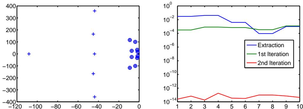
Figure 4: Power plant example from [7]. *Left plot:* Location of eigenvalues (crosses) and selected eigenvalues (circles). *Right plot:* Absolute error of the 10 selected eigenvalues after (i) extraction from the linearization, (ii) 1 Newton iteration, (iii) 2 Newton iterations.
