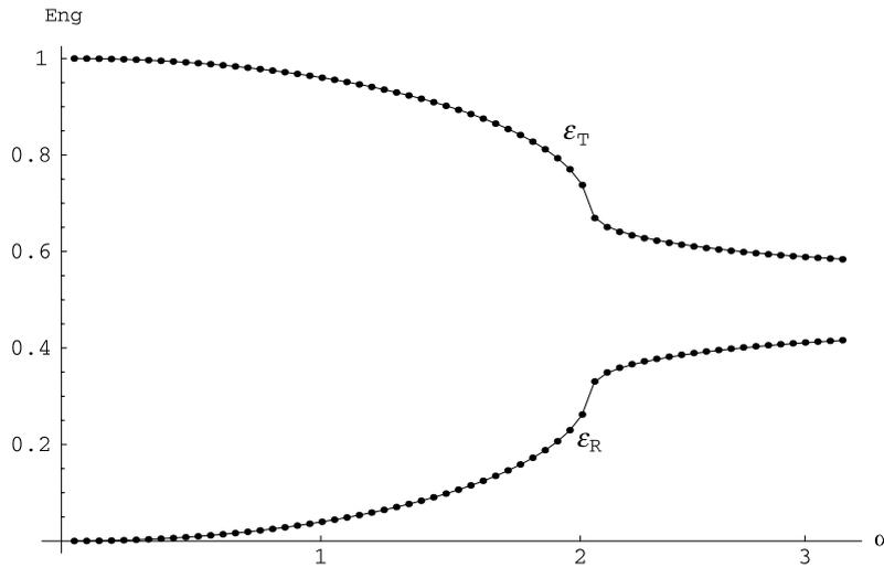
Fig. 13. Comparison of results for transmitted and reflected wave fields from Porter & Evans [19] (dotted lines) and from the exact result using the Wiener–Hopf technique (continuous lines) for  $\theta = 30^\circ$ . Comparison of results to those of Porter and Evans.
