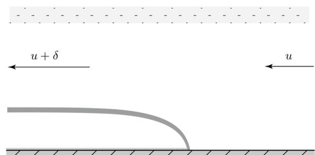
Figure 1: An illustration of the blocking effect of a fire-plume with vertical displacement of the flow restricted by a stably stratified atmosphere. The horizontal wind speed increases by an amount  $\delta$  from its incoming value of  $u$ . The fire is taken to be moving into unburnt vegetation on the left.
