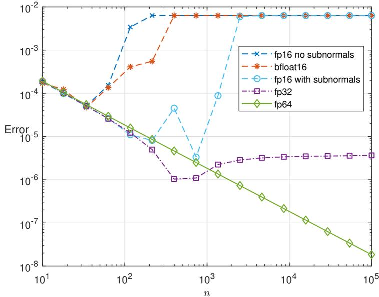
FIGURE 6.1. Absolute errors in Euler’s method for  $y' = -y$ ,  $y(0) = 0.01$ , over  $[0, 1]$ , in different simulated arithmetics, with stepsize  $h = 1/n$ .
