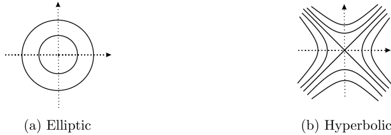
Figure 4.1: Curves on which the period of the symmetric periodic orbits is constant.
