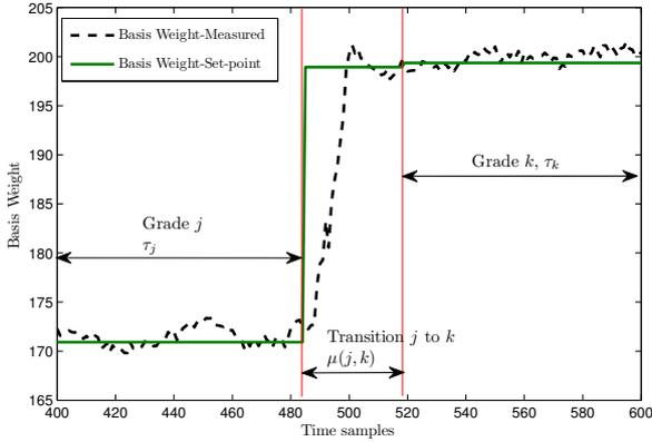
Fig. 2. Illustration of a grade change and associated times
