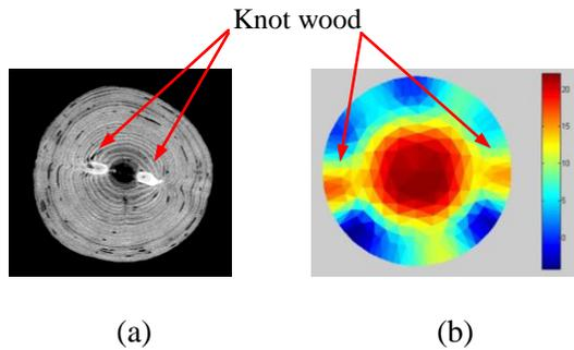
**Figure 5:** Cross-sectional CT (a) and TLDD (b) images showing knot wood.
