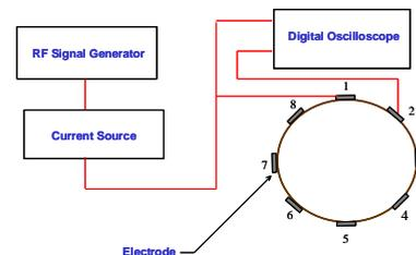
**Figure 2:** Block diagram of the TLDD scanning system.
