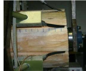
**Figure 1:** Photo of brush electrodes in the TLDD scanning system.
