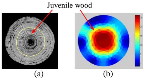
**Figure 3:** Cross-sectional CT (a) and TLDD (b) images showing the method for outlining juvenile wood.
